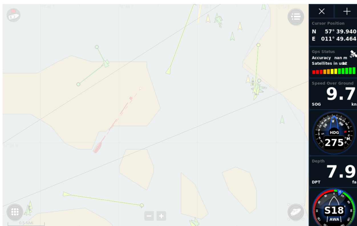
The Instruments Bar (right) providing persistent sensor data over a chart canvas.
